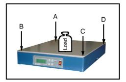
**Weight** shows the load on each corner. A flashing bar means an overload or bad load distribution, the system will not isolate.
