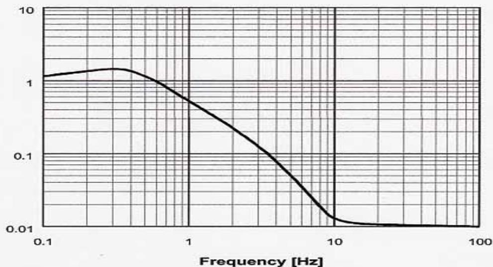
*Isolation:* dynamic 0.7 Hz to 1000 Hz, passive beyond 1000 Hz.
